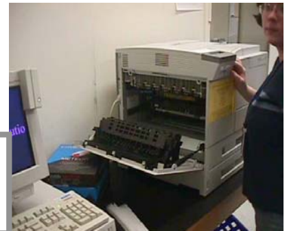
Left access door (fuser assembly) Caution – HOT!
